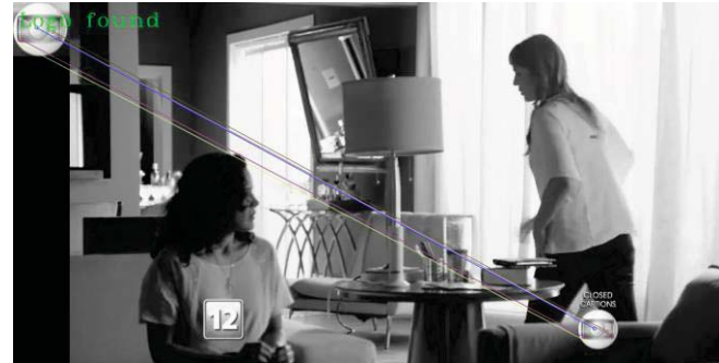
Fig. 2. Example of TV logo detection with \tau (distance ratio) parameter equal to 0.95
