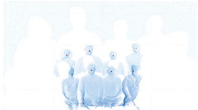
Fig. 7: In this point cloud image, eight people were captured. Our face detection approach is successfully detecting seven faces and one is missed.
