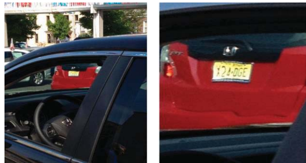
Figure 1. The defective car windshield images with transmitted distortion defects.
