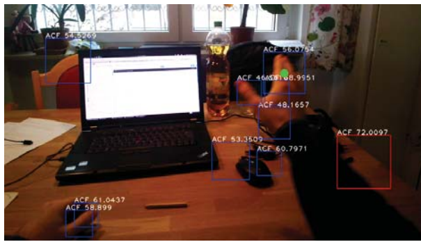
(c) Correct hand position not under the ten best candidates. But at least some candidates are on the hand and their scores are above 45. The best candidate at the right table margin has a score of 72. The candidates close to the computer mouse have scores between 53 and 60.
