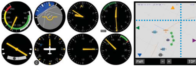
Figure 8: Virtual instrument panel and control indicator
