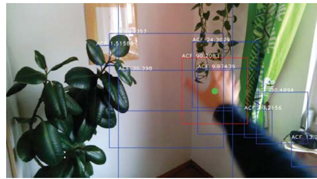
(d) Hands are even detected at the wall but the correct hand location has the best score with 90 compared to 30 of the second best candidate.
