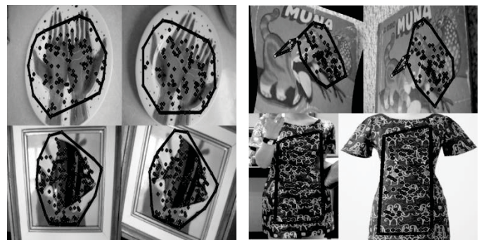
Figure 2. Matching results for clustering of geometric similarity. (left) Perspective transformation, (right) deformable transformation
