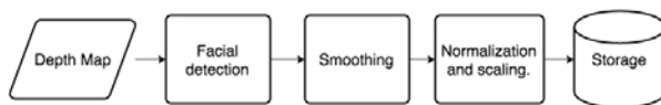
Figure 3. Once a face is detected, the facial area is stored as a face image and then smoothed, normalised and scaled before being stored.
