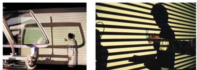
Figure 2. Current inspection tasks by human visual judgment and the testing images with transmission of standard patterns.
