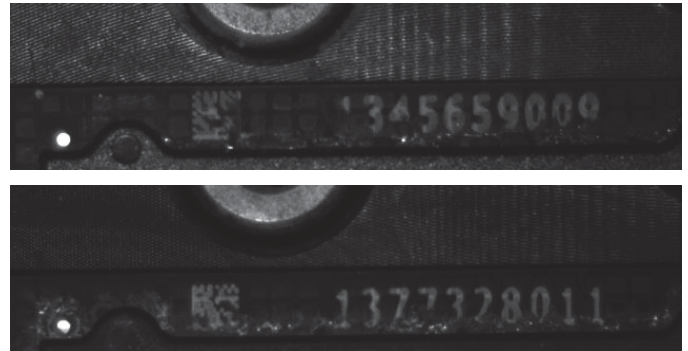
Fig. 2. PCBs with evident residual dirt over characters.
