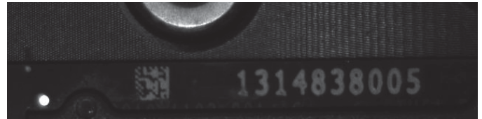
Fig. 1. PCB with no damaged characters.
