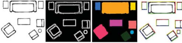
Fig. 10: Outputs after performing different steps of image segmentation on conversation area image.
