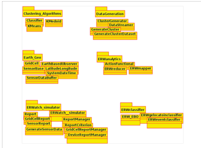
Figure 9: Primary software packages and the major C++ classes they contain. These depend on custom math and statistics packages developed for this project. The latter packages (not shown) constituted a major portion of the code.
