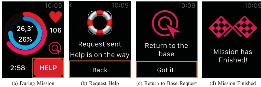
Fig. 4: Smart Watch Application: shows the main Watch UI screens. During the mission the worker can view different quantities such as humidity, temperature inside the suit, the heart rate and the elapsed time. The participant can ask for help using the help button. Request help shows the screen when the worker requested help. Return to Base shows the UI as soon as the Commander requested a return. As soon as the worker returned to the secure zone the mission finished screen is shown. All buttons are highlighted with an orange border.
