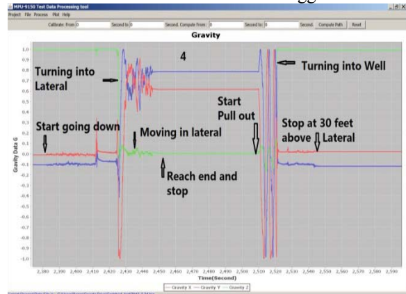
Figure 12. Zoomed portion focusing on the fourth test run in figure 11. It can clearly be seen when the sensor turns from vertical to horizontal and when the sensor is stationary or moving.
