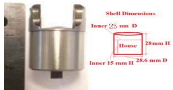
Figure 1. Steel Shell and its dimensions and ledge
