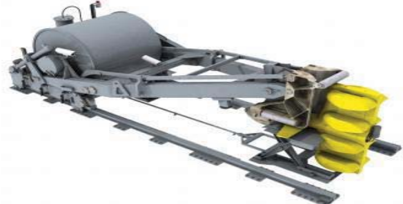
Fig. 4 Overboarding unit of CAPTAS [3]
