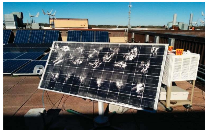
Figure 1. The PV panel with levels of treatments. The tilt at 60°, the panel toward the south, the wind at 0, and low level of cleanness.
