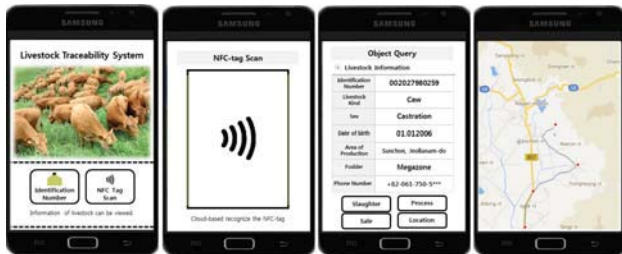
Fig. 6. Mobile Application for Livestock Traceability Management System
