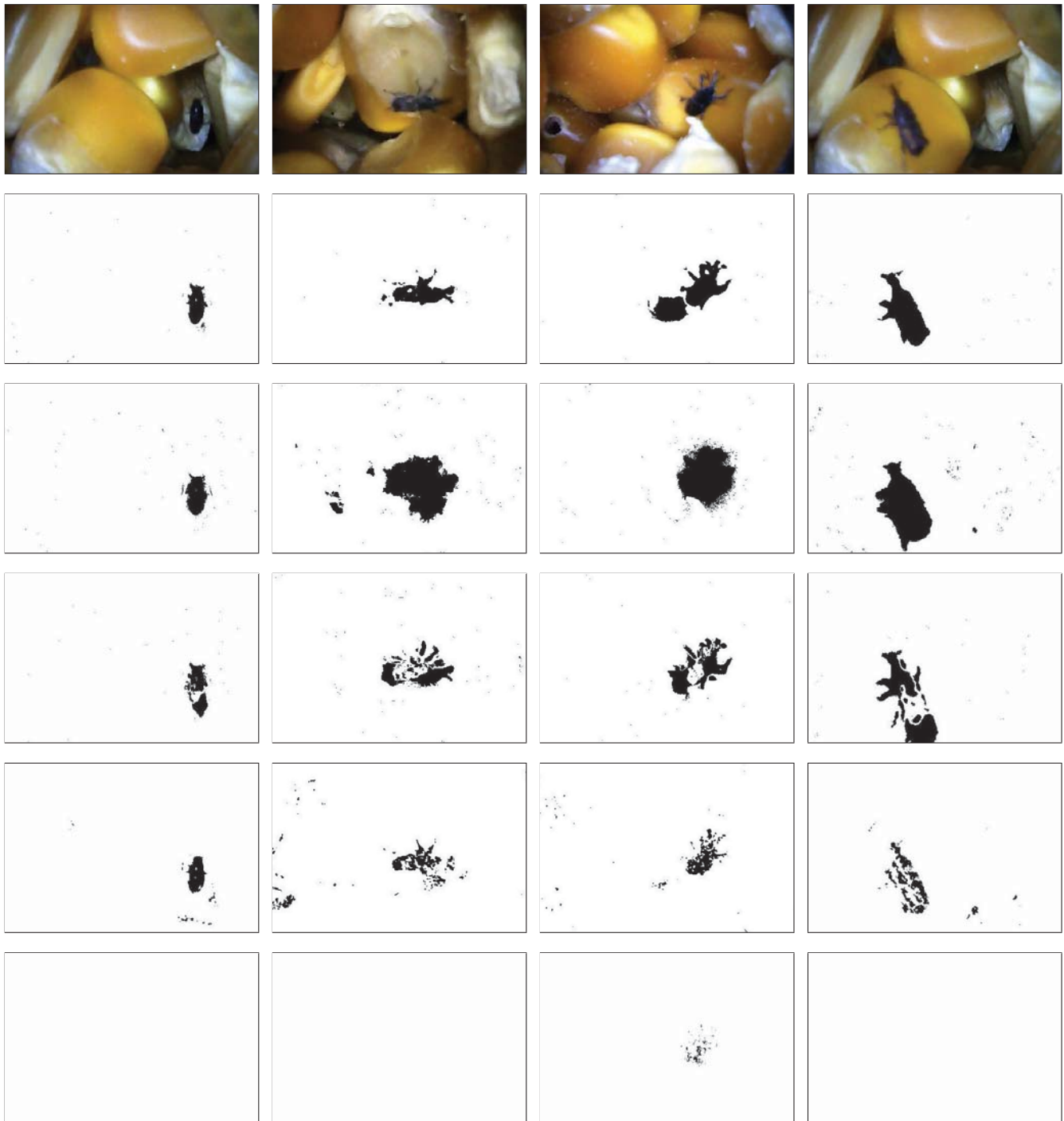
Fig. 6: This Fig. is a continuation of Fig. 5. Original images in the first row and Result obtained by the methods analysed: second row – DPWrenGABGS; third row – DPEigenbackgroundBGS; fourth row – AdaptiveBackgroundLearning; fifth row – FuzzyChoquetIntegral; sixth row – T2FGMM_UM. The settings of each algorithm are given in the Table 1.
