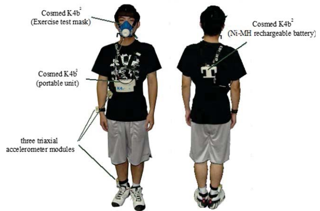
Fig. 1. A participant wears K4b 2 and the wearable physical activity sensor system. (a) The front view of the participant. (b) The back view of the participant.
