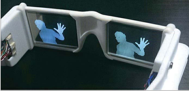
Figure 5. Experimental prototype of 'smart glasses' to enhance vision for poorly sighted individuals. This system has a see-through display and a special type of camera that can detect and highlight nearby objects [60].
