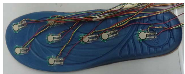
Fig. 4 Insole with embedded sensors.
