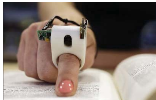
Figure 4. The FingerReader device [58] for reading printed text (image courtesy of [59])
