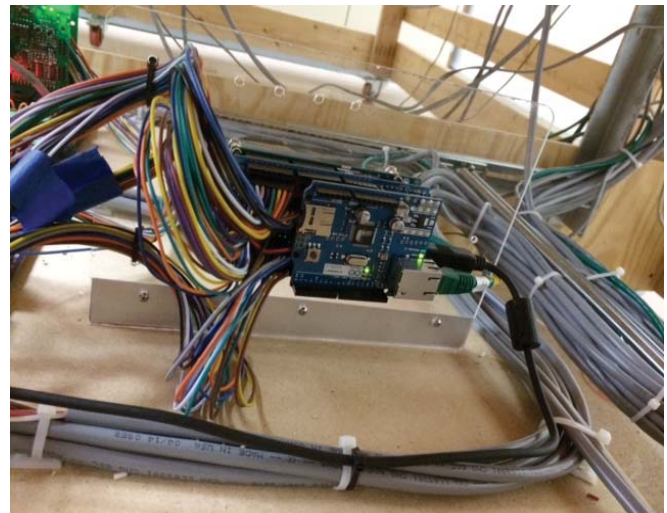
Figure 5 – Photo of Arduino-based safety monitoring system
