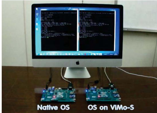
Figure 4. Test environment: native OS vs. OS on ViMo-S
