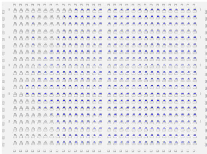
Fig. 4. Xilinx Spartan 2 CLBs layout
